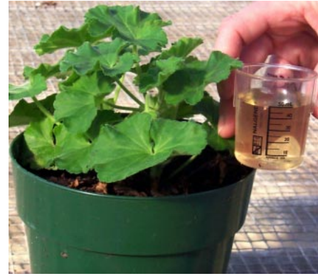
Figure 2f. Collect 50 ml (1.5 ounces) for testing.
