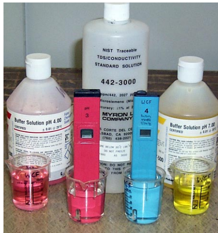
Figure 2g. Calibration standards for testing.
